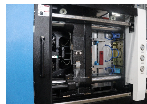
加大顶出力和顶出行程，适应瓶坯的顶出要求 Increasing ejector force and ejector stroke, adapts with PET preform drawing
